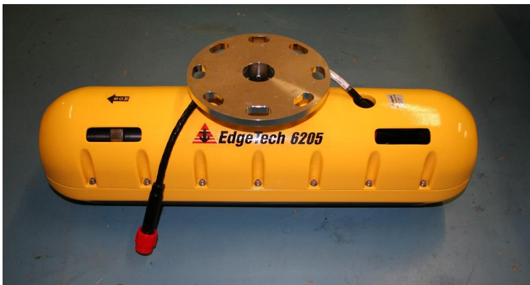
Figure 2-16: Array Replacement Complete
