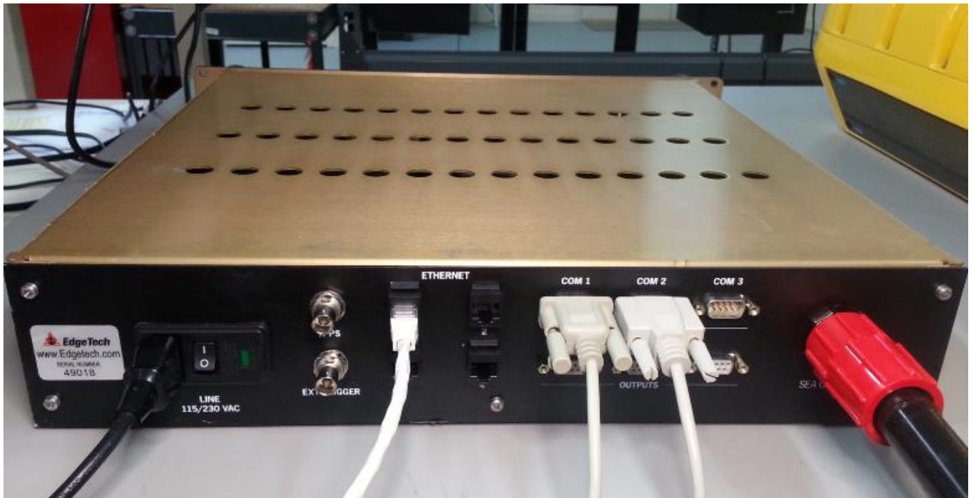
Figure 2-17: Rack Mount Topside with Real Time Connections
