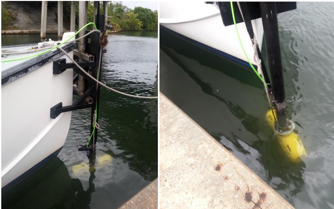
Figure 4-1: 6205 Deployment, Option 1 – Over-the-Bow
