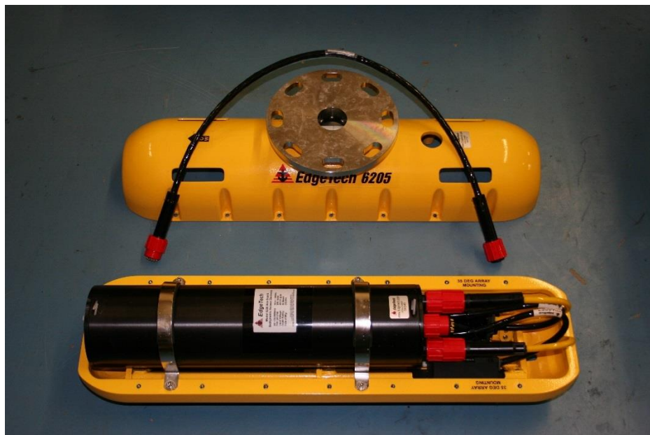
Figure 2-8: Top Housing and Deck Cable Removed
