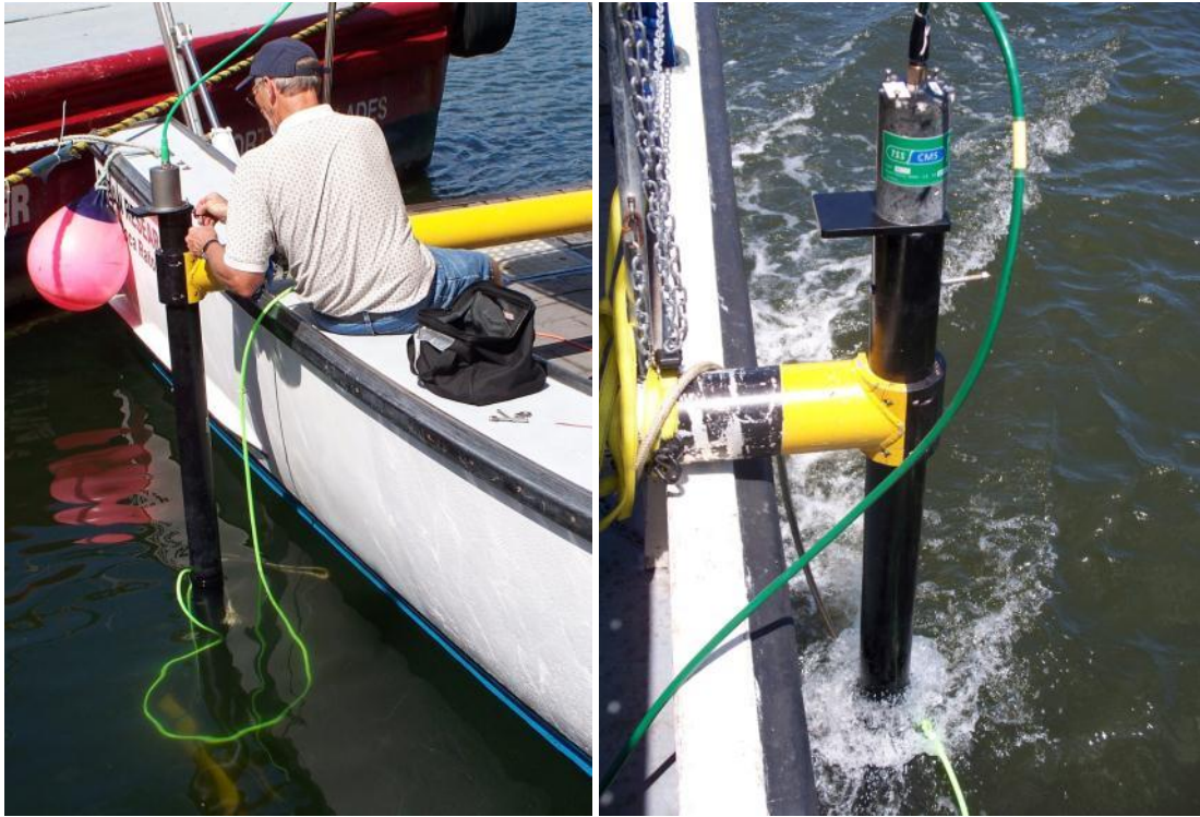
Figure 4-2: 6205 Deployment, Option 2 – Over-the-Side
