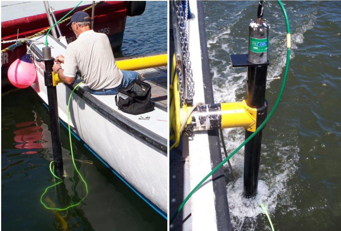
Figure 5-2: 6205s Deployment, Option 2 – Over-the-Side
