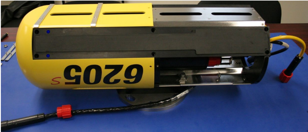
Figure 5-11: All Cap Screws Removed
