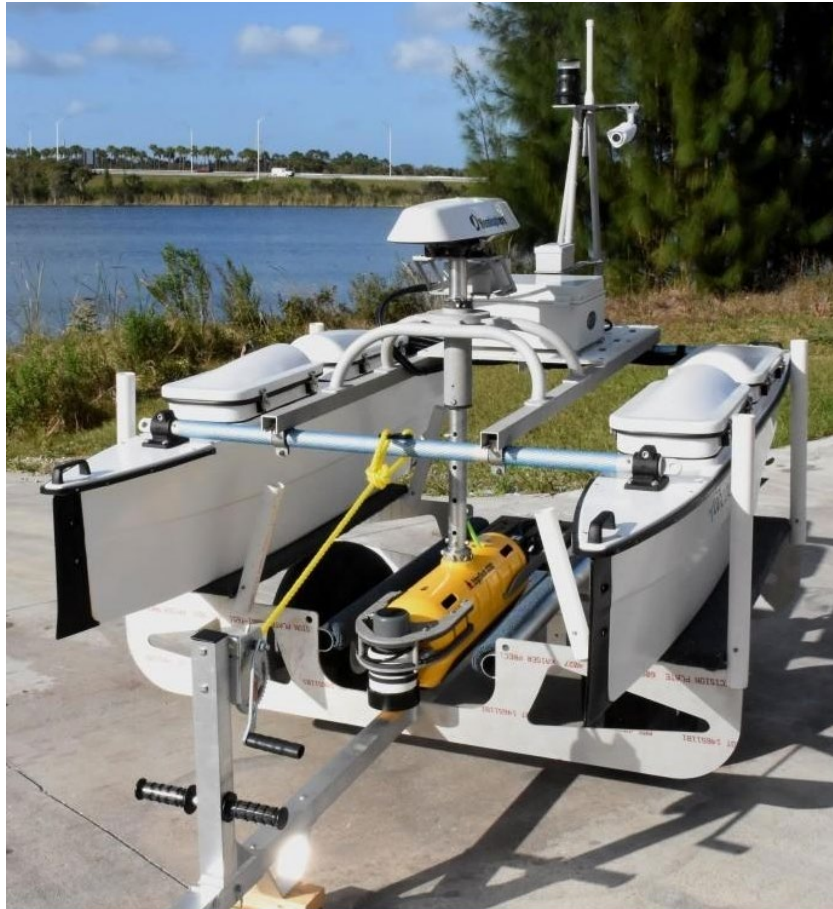
Figure 5-3: 6205s Deployment, Option 3 – to a USV (Sea Robotics in this example)
