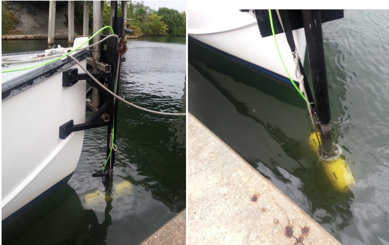
Figure 5-1: 6205s Deployment, Option 1 – Over-the-Bow
