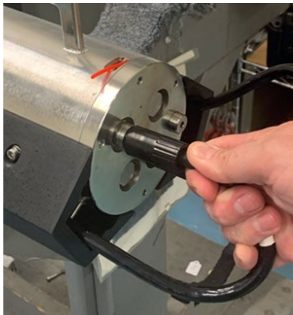
Figure 7-2: Aft Endcap Cable Disconnection
