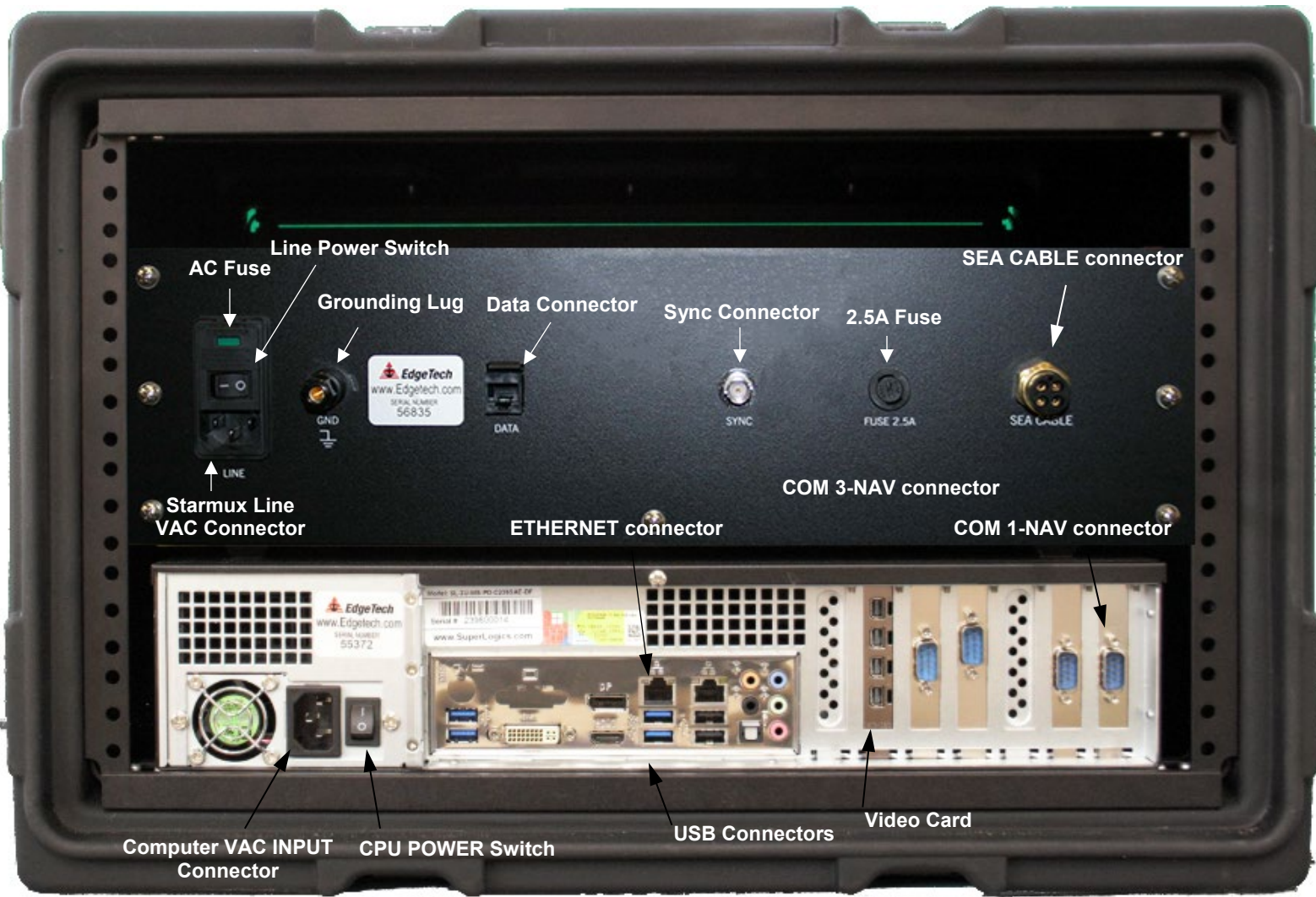
Figure 3-10: 4205 Starmux III Rack Mount Topside Processor Rear Panel
