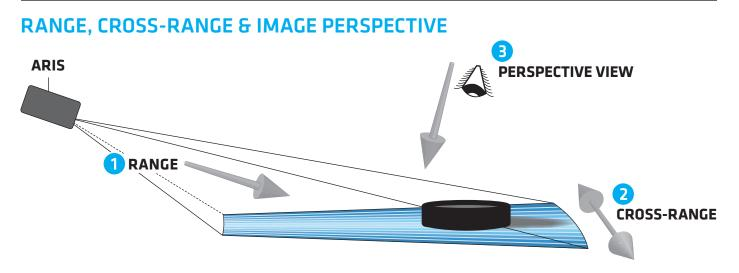
Range, cross-range, and perspective are relative to the acoustic wedge. Each of these are at 90° to the other two, much like three edges that come together at the corner of a box.
