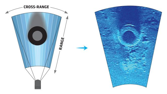
The following illustrations demonstrate how to image an object lying on a surface using the ARIS Explorer:
