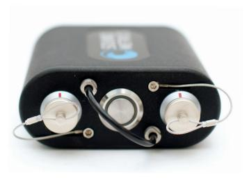
The Command Module monitors the power and connection status of the sonar. The ring-shaped LED around the main power switch gives visual feedback on the current operating state of the system.
