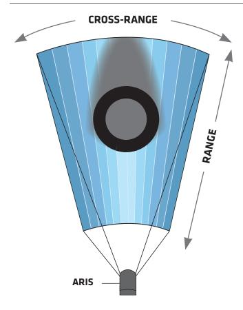
Multiple beams directed from the ARIS Explorer create a fan of narrow slices that form the "acoustic wedge." Each individual slice produces a section of the image, where information in range is then placed appropriately with neighboring information in cross-range to produce the entire image.
