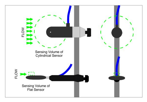
The sensor should be aligned into the flow and the calibration is determined for +ve flow [flow on to the sensor at the electrode end] with the sensor upstream of the wading rod.
