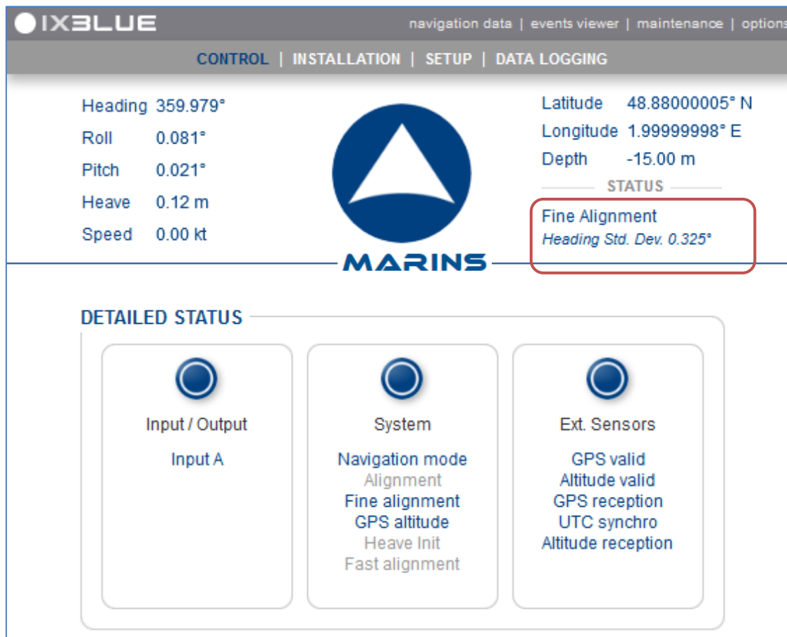
Figure 8 - Web-based User Interface during the fine alignment (there is no 'Fine alignment' flag for QUADRANS)
