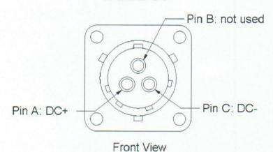
Bulkhead Connector: MS3470L12-3PY Mating Cable End: MS3476L12-3SY (or equivalent)
