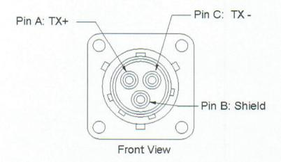
Bulkhead Connector: MS3470L12-3S Mating Cable End: MS3476L12-3P (or equivalent)
