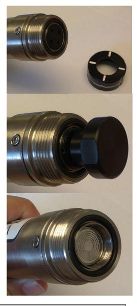
Any damage to this diaphragm will render the instrument warranty invalid.
