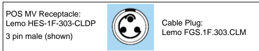
Figure 10: PWR Connector Pin Arrangement
