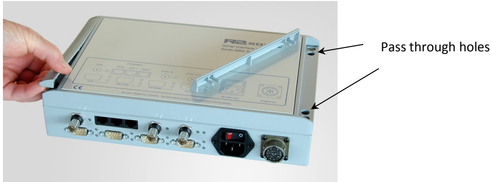
Figure 35: Removal of trim to expose securing holes
