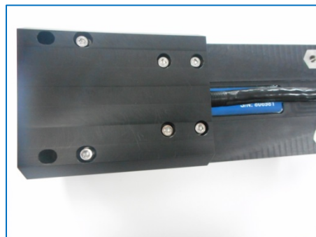
Figure 21: Projector cable clamp in place
