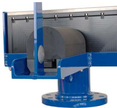
Figure 28: View of the mounted Projector; NB. Connector is facing protective fin
