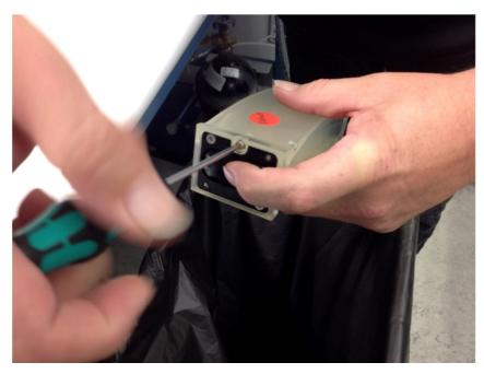
4) Holding the lens at an angle of about 30° over a container that can collect any spilled lens fluid, back out the vent plug most of the way (but do not remove) on the end where the black plastic protective cover has been removed.
