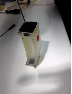
3) Remove the black plastic protective cover from one end of the lens with the 2mm hex driver. Replace the 2 screws to better secure the diaphragm after removing the black plastic protective cover.
