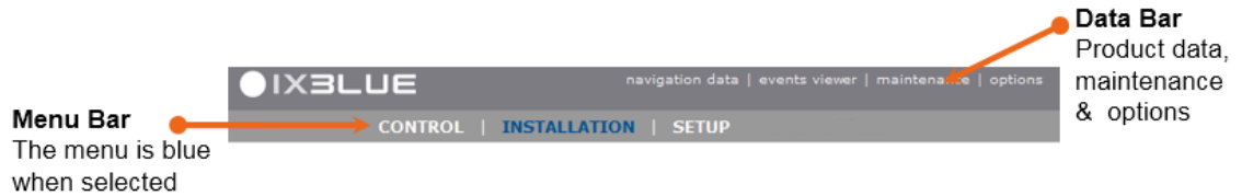
Figure 9 - Menus of the Web-Based Graphical User Interface
