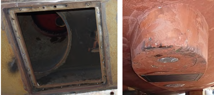
Sea chest with flange, threaded holes and the two (bigger) water inlet holes prepared by the ship yard (left) and transducer mounted into a dome/blister to prevent air bubbles washed below the transducer (right).
