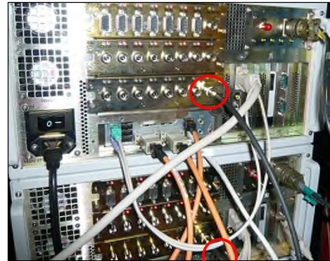
Trigger OUT connectors at SeaBat 7125 topside units (BNC connectors at rear panel)
