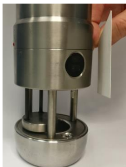
In air test of Turbidity Sensor
