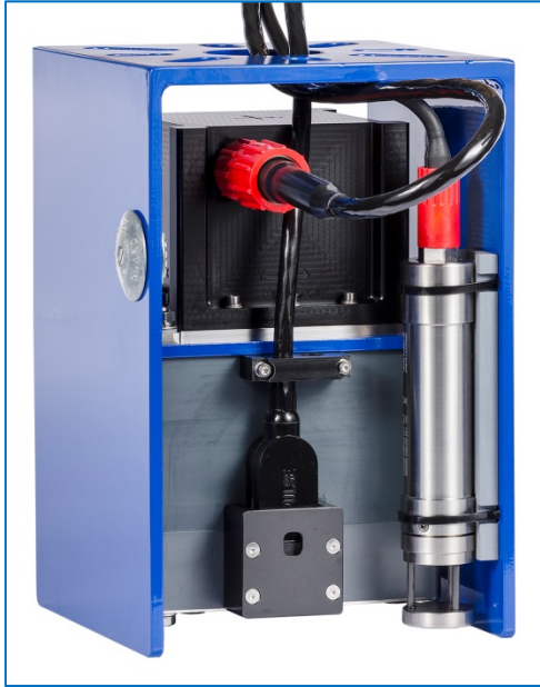
Figure 119: Aft detail of the IMU cable connection
