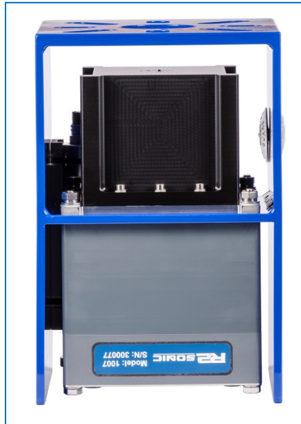
Figure 117: IMU mounted within the Sonic 2022 mounting frame
