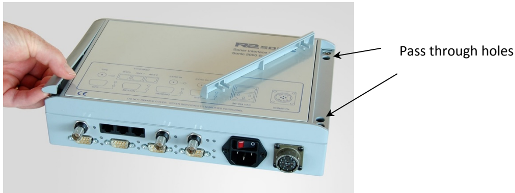
Figure 12: Removal of trim to expose securing holes
