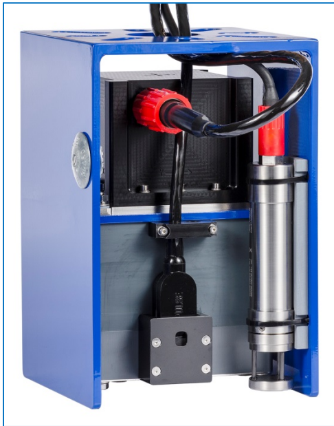
Figure 119: Aft detail of the IMU cable connection
