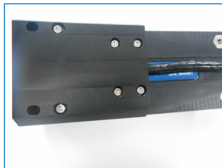
Figure 21: Projector cable clamp in place
