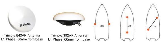
The Primary Antenna (Antenna 1) should be nearest to the IMU so that offset measurement errors are minimized. The Secondary Antenna (Antenna 2) should be a fixed distance from Antenna 1. It is recommended that the antennas be at least 2m apart. The antennas should be positioned parallel to the water surface to within 2-3cm.
