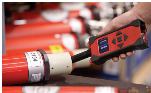
Figure 5-2 – Positioning the iWAND Against the Instrument Transducer
